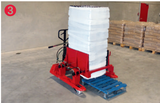
The defective pallet is unloaded with a free lift and then replaced by a tradeable DHP.
