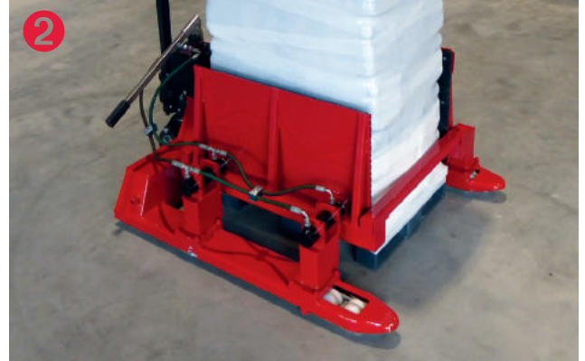
The goods are picked up via the hydraulic clamping and lifted from the pallet via HUBI.
