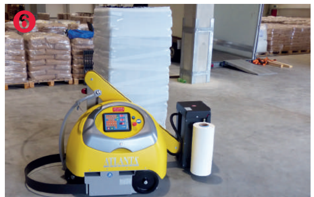
After 2 to 4 windings at the pallet foot the pallet is again save for loading and ready for transport. Done! Thanks to HUBI the pallet exchange only takes 5 minutes.
